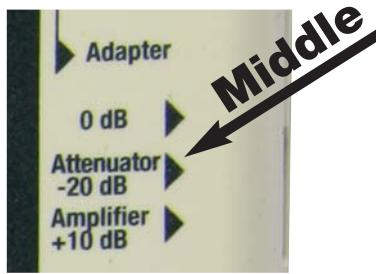
When the attenuator is connected, set the "Adapter" switch of the HF-Analyzer to "Attenuator -20 dB" (See picture on left). This activates the integrated automatic conversion feature of the HF-Analyzer. The true signal strength value can be read from the display without any manipulation. The vertical line on the left side of the display indicates the correct measuring unit.
