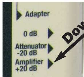
When the preamplifier is connected, set the "Adapter" switch of the HF-Analyzer to "Amplifier +20dB" (See picture on left). This activates the integrated automatic conversion feature of the HF-Analyzer. The true signal strength value can be read from the display without any manipulation. The vertical line on the left side of the display indicates the correct measuring unit.
